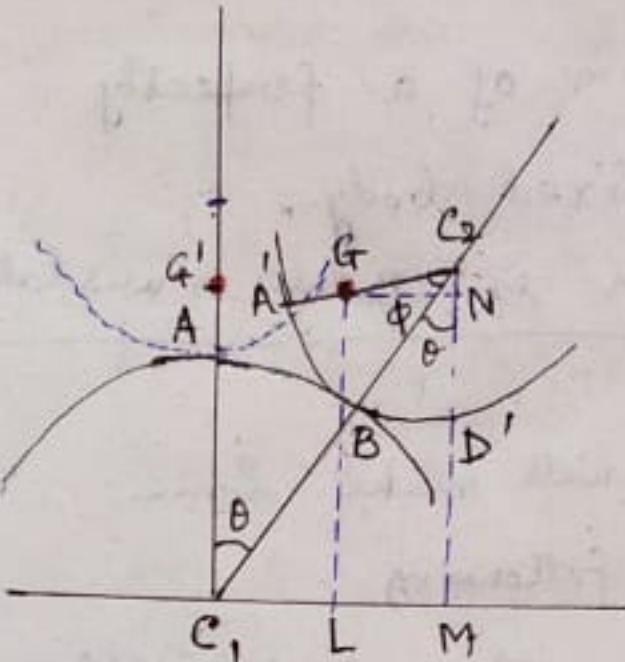
The upper body is kept in equilibrium by two forces acting on it, viz., its weight acting vertically downwards through its centre of gravity and the total reaction at the point of contact; it follows that the c.g. is on the vertical through the point of contact.
