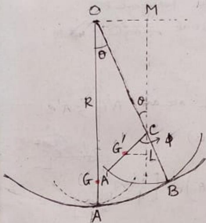
As before the upper body is kept in equilibrium by the action of two forces on it, viz., its weight acting vertically downwards through its centre of gravity and the total reaction at the point of contact.
