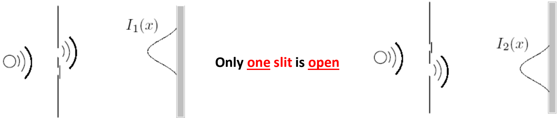
Fig: Curves I(x) give the intensities of the waves passing through slit and reaching the screen at x .
